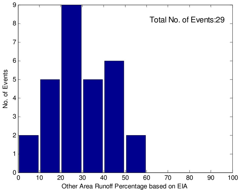
**Figure 8-7. Powells Creek (NSW) - Histogram of Identified Storm Events – Volume of Runoff from Other Area relative to total runoff**
