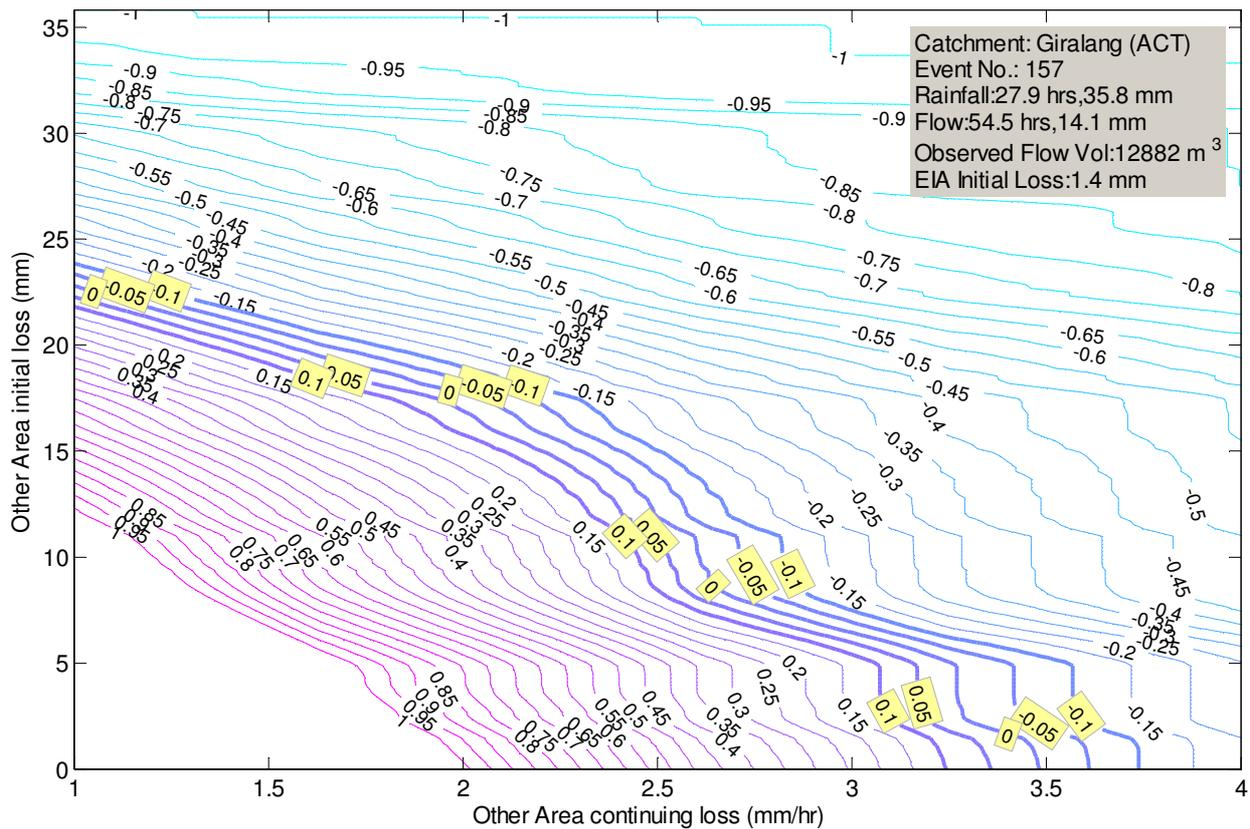
**Figure 7-2 Error contours for different Initial Loss – Continuing Loss pairs for the Other Area. The Error is defined as (Simulated Runoff Volume – Observed Runoff Volume)/(Observed Runoff Volume – EIA Runoff Volume).**
