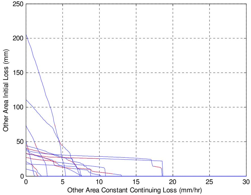
Figure 9-5. Contour Plot of Initial Loss & Constant Continuing Loss – PowellsCk (NSW)
