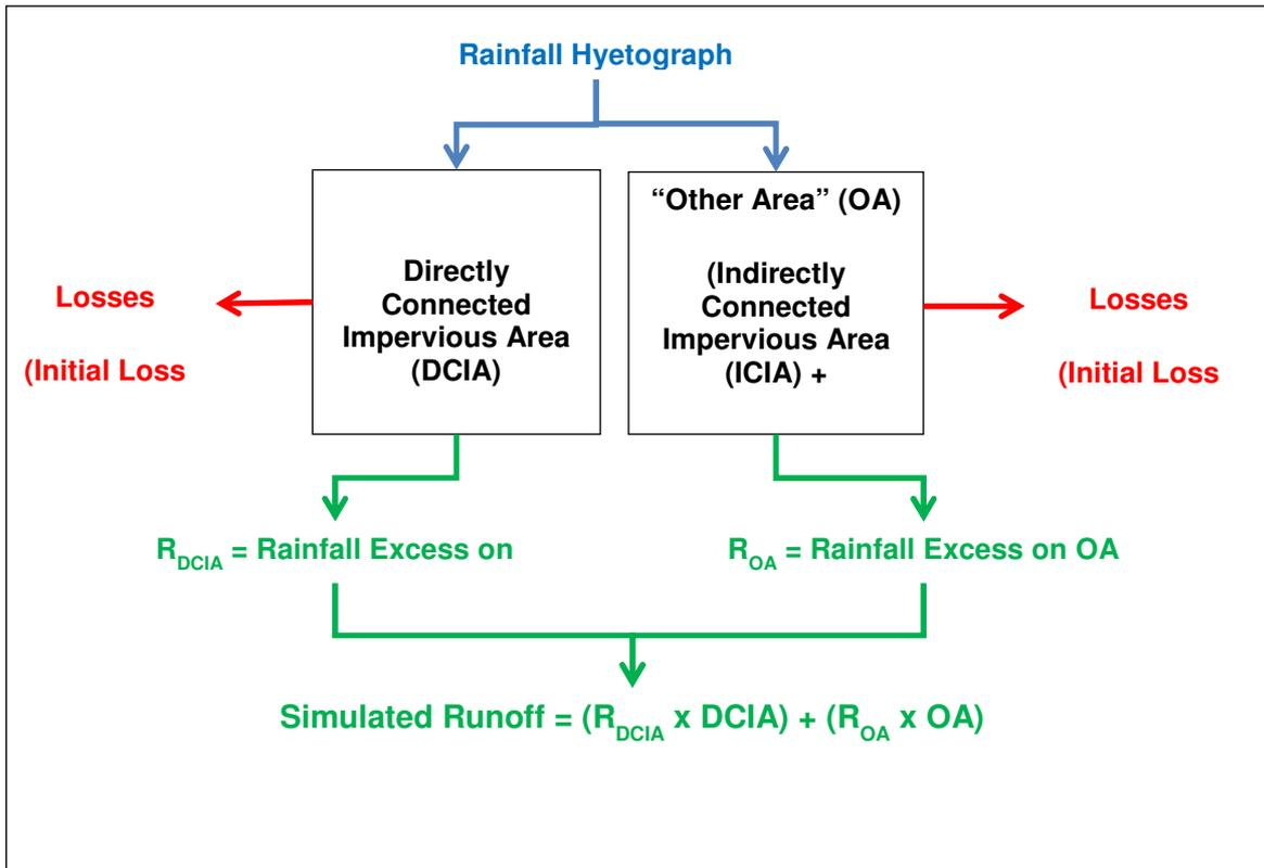
**Figure 7-1 Methodology to determine losses based on volumetric analysis of historical storm events**
