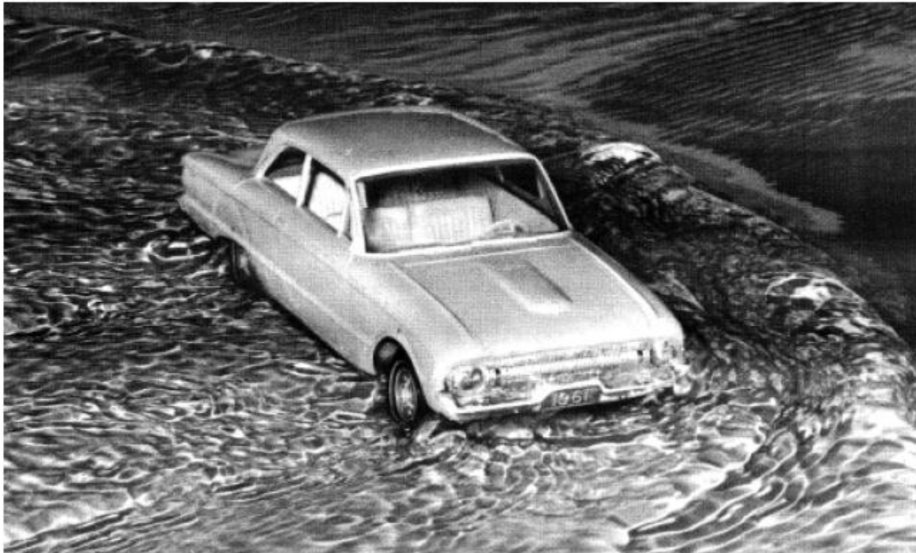
Figure 4 Model Ford Falcon at 1:25 scale used by Bonham and Hattersley (1967)
