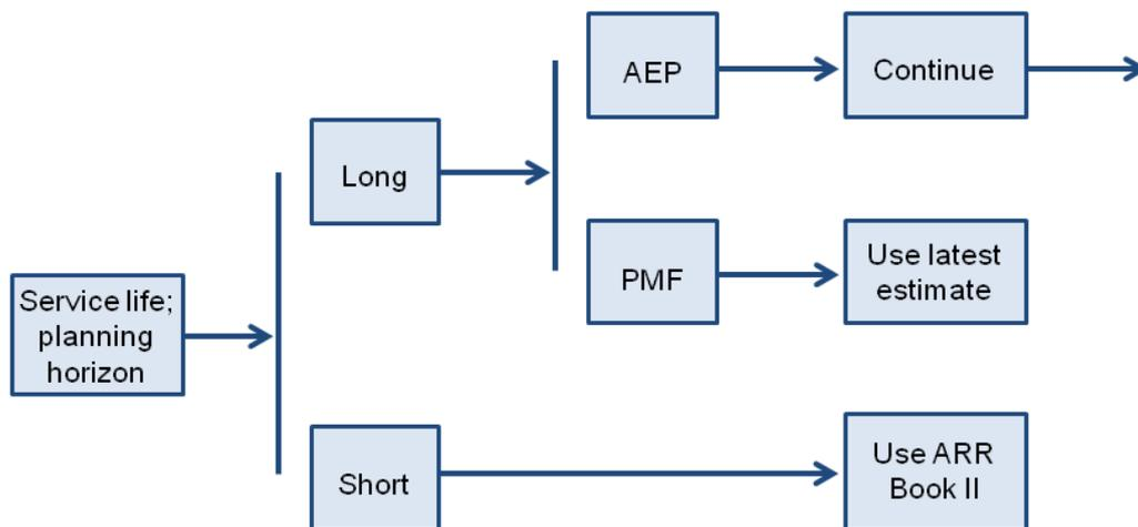
**Figure 2 Decision tree for incorporating climate change in flood design – Part 1 of 3 (AEP = annual exceedance probability; PMF = probable maximum flood; ARR Book II = design rainfall intensity (or equivalent depth) for current-climate conditions)**
