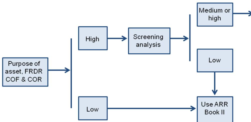
**Figure 3 Decision tree for incorporating climate change in flood design – Part 2 of 3 (FRDR = flood-related design requirements; COF = consequences of failure; COR = cost of retrofits; ARR Book II = design rainfall intensity (or equivalent depth) for current-climate conditions)**
