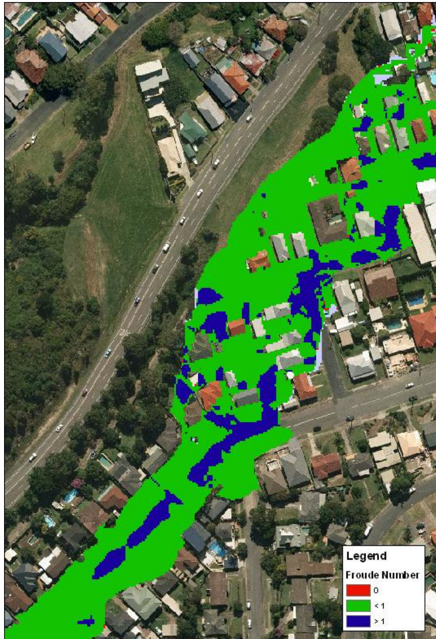
Figure 29: Numerical Model: Froude Number Analysis for the Merewether floodplain with Buildings
