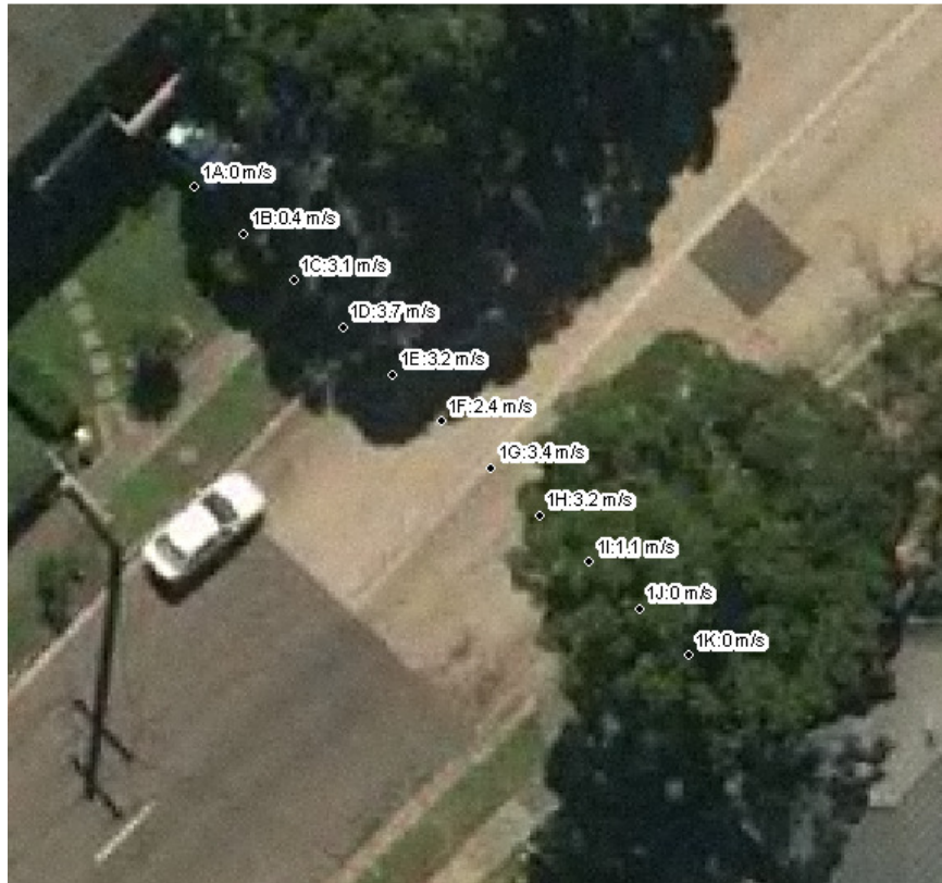
Figure A1: Velocity Measurements: Transect 1
