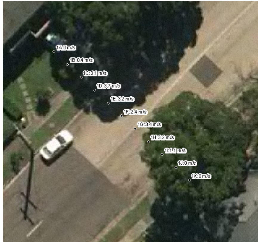
Figure 20: Velocity Measurements: Transect 1
